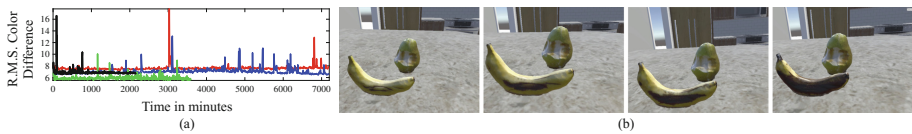
Fig. 8. (a) Plot of root-mean-square (r.m.s.) frame-to-frame appearance difference against time. (b) Frames showing interactions with a VR environment containing spatiotemporal 3D models. The user plays forward aging in the banana and pear.
