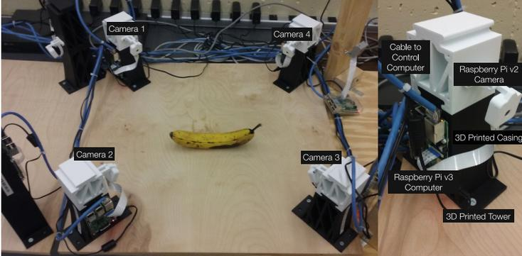
**Fig. 1.** Microenvironment to capture multi-view time-lapse images consisting of four Raspberry Pi v2 cameras connected to four Raspberry Pi v3 computers.
